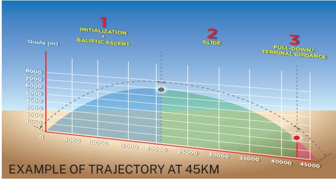
The flight sequences of the Vulcano 127mm ammunition encompass a Ballistic Flight Path (1) involving initialization and GPS acquisition, a Glide Path (2) with Mid-Course Navigation and Terminal Guidance (3) with GPS or IR or SAL mode, depending on the configuration.
