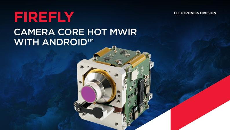
The Firefly Camera Core uses a high operating temperature (HOT) Mercury Cadmium Telluride (MCT) array with a resolution of 640 x 512 pixels on a 16µm pitch. Firefly provides all of the processing and interface requirements to drive a multi-functional hand held thermal imager, including additional camera channels, combined into an infrared camera core.
