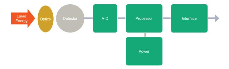
The GEN III SAL seeker detects the pulsed laser signal within the field of view. The laser signal is processed to determine if the correct code is received e.g. NATO STANAG 3733 and its bearing relative to the seeker boresight is calculated. For non-NATO users, other country specific PRF codes can be utilised. The target bearing is reported to the host weapon via the RS422 communication link.
