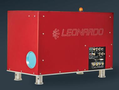
Leonardo's homogenized pump engine has a modular internal design that can be custom-configured to meet your requirements. Pulsed and CW operation, wavelengths ranging from 760 nm-1100 nm or 1400 nm-1700 nm, rectangular or hexagonal output beam shape, different beam sizes, and different integration levels are just some of the factors that can be adjusted.
