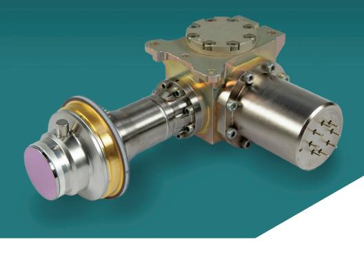
The SuperHawk infrared detector is a 1280 x 1024 array of pixels on an 8µm pitch, manufactured using a Metal Organic Vapour Phase Epitaxy (MOVPE) process with Mercury Cadmium Telluride (MCT) detector material grown on low cost substrates.
