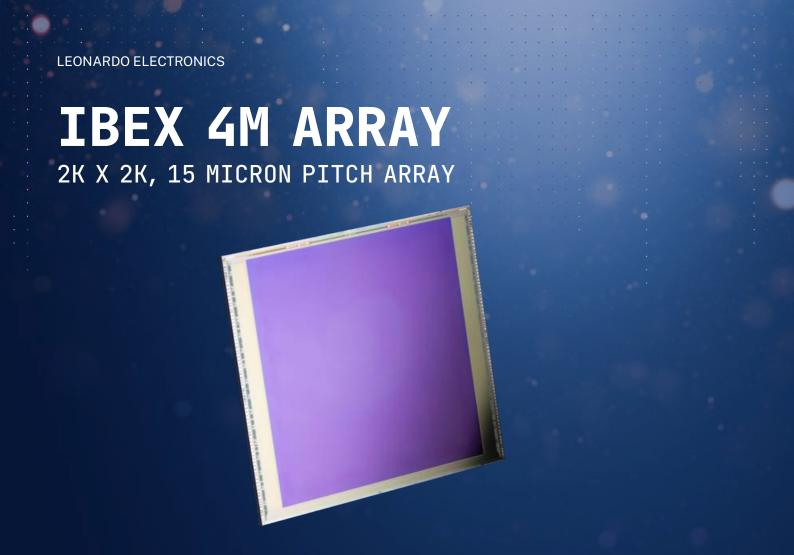
The IBEX 4M array from Leonardo is a  $2k \times 2k$ , 15 micron pitch array designed for use with designed to accommodate Leonardo's avalanche Photo-diode MCT structure. The design incorporates a number of features including flexible scanning and reference pixels as well as glow suppression. In addition, it has design features for enhanced radiation hardness. For extra flexibility, there is an option for 4, 8 or 16 output buffers.
